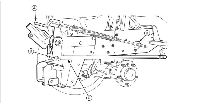
Figure 11. Lift Linkage Installation
